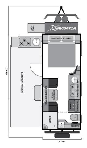
SIZE CLOSED - INCLUDES A/C Length 7.55m - Width 2.35m - Height 3.1m
